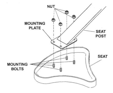
**4.** Place SEAT upside down and remove NUTS on MOUNTING BOLTS. Lower MOUNTING PLATE of SEAT POST down onto MOUNTING BOLTS and fasten with removed NUTS.
